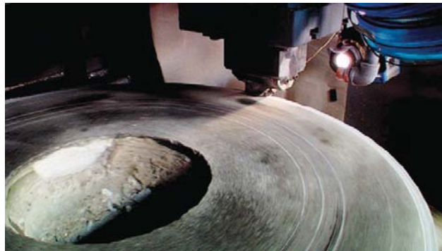
Figure 2.23: Face turning of rock with a single PDC cutter on a VTL (Bellin et al., 2010).
