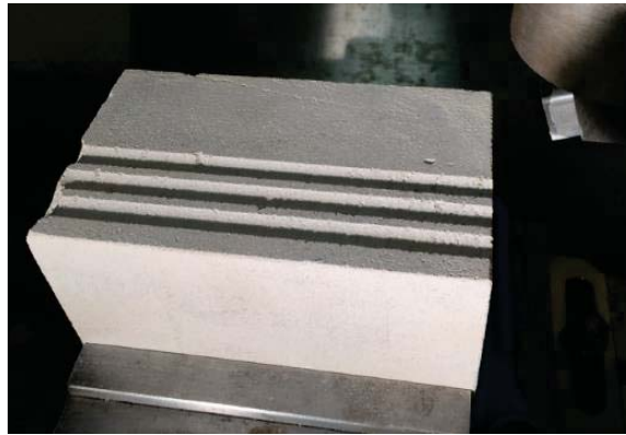
Figure 5.6: Indiana limestone sample after three repeated cutting tests.
